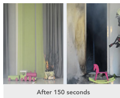
Comparative burn test: This test shows how flame retardant Trevira CS textiles (left) melt away once the ignition source has been extinguished, while conventional fabrics go completely up in flames.
