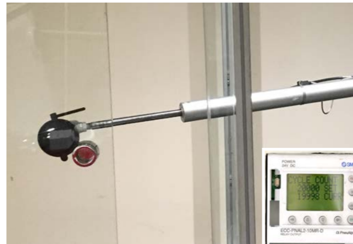
ENDURANCE TEST The shower door is open and closed on a 20,000 cycle to ensure endurance.
