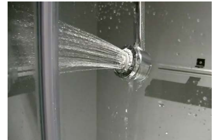
WATER RETENTION TEST High pressure shower is directed at the door to ensure there's no leakage.
