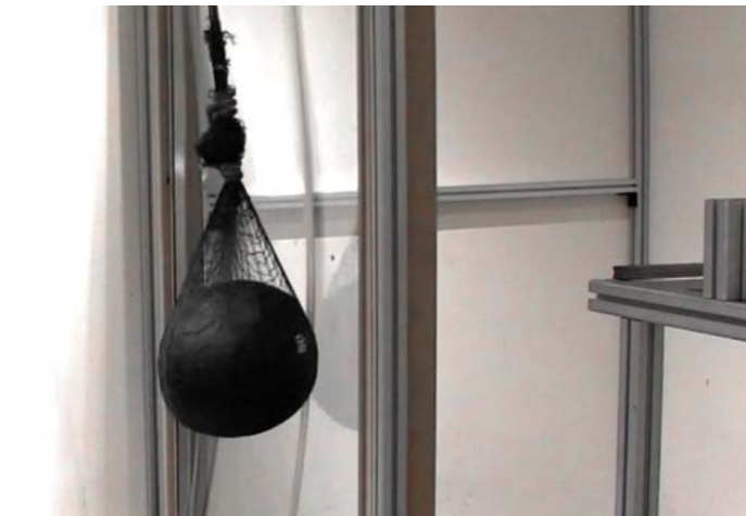
STRUCTURAL STABILITY TEST A ball up to the weight of 50kg is launched into the enclosure to ensure rigidity if there is a fall.
