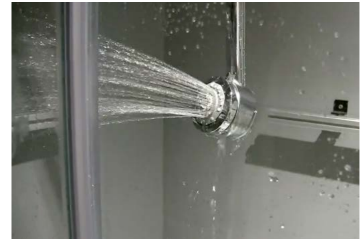
WATER RETENTION TEST High pressure shower is directed at the door to ensure there's no leakage.
