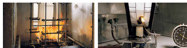
In the important international burn tests Trevira CS Bioactive counts as flame retardant. Above, the stringent test to DIN 4102, Class B1, and the French "Brûleur électrique", one of the hardest tests worldwide.
