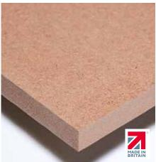
Kronobuild® FR MDF are non-load-bearing boards with improved fire retardant properties and are manufactured in compliance with European standard EN 622-5 where they are defined as boards for general use in dry conditions. FR MDF is increasingly used particularly in public spaces where stringent fire regulations must be met. According to EN 13501-1 boards are classified B-s2, d0 in terms of reaction to fire.
