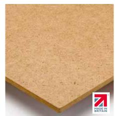
Kronobuild® HDF is an engineered board produced from resin bonded wood fibres under high pressure and heat. HDF is a non-loadbearing product for interior use in dry conditions. Due to its very fine unsanded surface, HDF is suitable for a variety of coatings; laminating, painting, varnishing and veneering.
